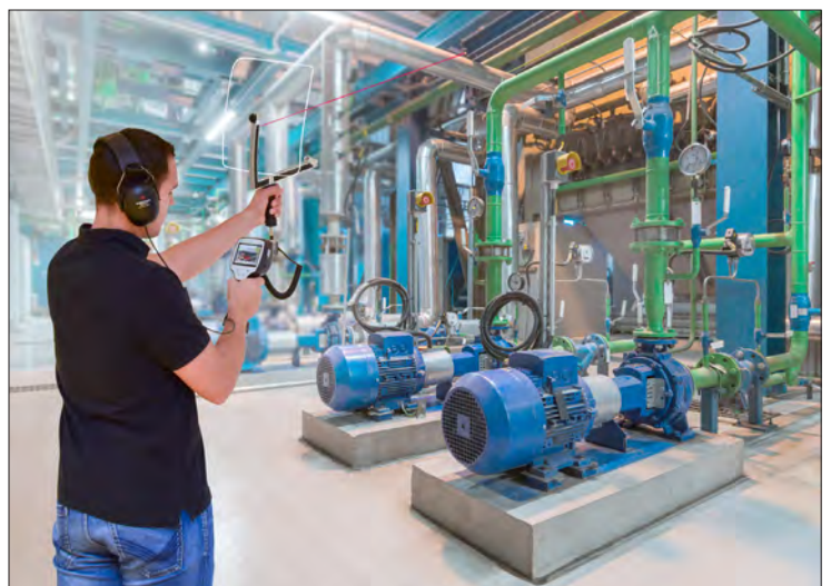
Accurate leak detection during operation with laser pointer and integrated camera
